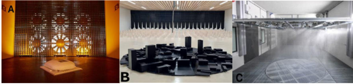
Figure 1. Infrastructure of the Wind Engineering Laboratory (LIW) and the Environmental Aerodynamics Laboratory (LAŚ) at the Cracow University of Technology planned for use in tests of the proposed aero-robotic inspection and repair system: A – the large-scale wind tunnel for snow engineering at LAŚ PK; B – the large-scale wind tunnel for building aerodynamics at LAŚ PK; C – the large-scale climatic wind tunnel at LAŚ PK.
