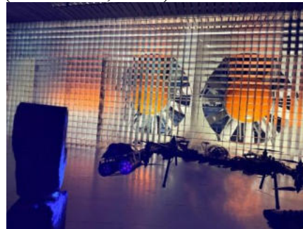
Figure 2. Example of the planned UAV test arrangement in the wind tunnel test section.
