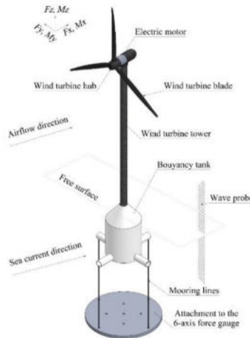
Figure 1. Model of the TLP OWT used for scaled experiments
