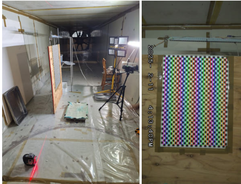
Figure 1. Experimental setup and image calibration procedure. (Left) Wind tunnel configuration showing the jet injection system, high-speed camera, lighting arrangement, and leveled calibration checkerboard used to establish the pixel-to-millimeter conversion. (Right) Raw image from the camera view, showing where the checkerboard pattern is automatically detected using OpenCV for spatial calibration.
