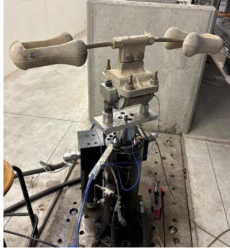
Figure 2. Stockbridge damper plus clamp mounted on the hydraulic actuator
