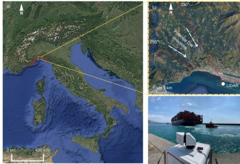
Figure 1. a) City of Genoa in the north-west of Italy, with the Liguria region indicated in red; b) position of the scanning LiDAR in the Port of Genoa, potential directions of DWs and the scanning path of the LiDAR during the measurement campaign; c) scanning LiDAR at the end of the quay.
