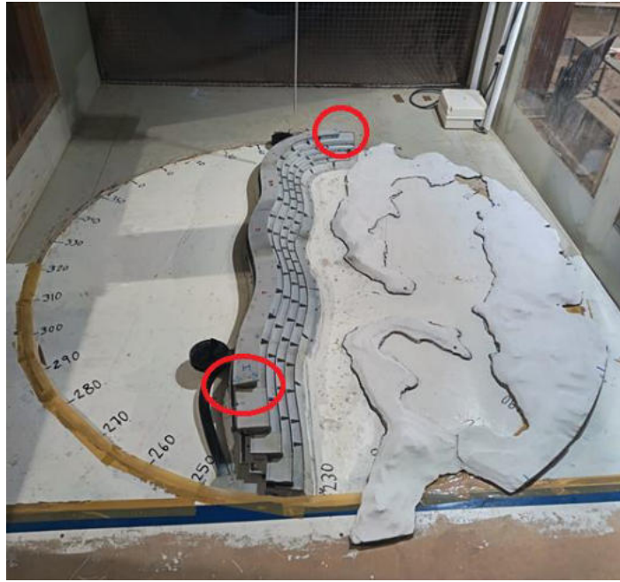
Figure 3. Model installed in UdelaR Wind Tunnel main testing section. In red areas were conical vortex develop
